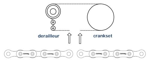
1. Insert one half of the Connex link into the end of the chain that comes from the chain ring.
