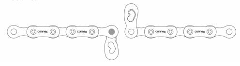
3. Position the chain ends on top of each other and insert the pins from each link into the corresponding receiving holes on the opposite link.
