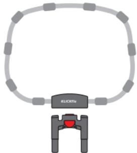
**Mounting** Use this coupling for KLICKfix handlebar adaptersystem only on original Reisenthel bikebaskets (5kg max.). Clip both parts in the middle onto the straight side of the aluminum bracket. Insert the 4 screws from below as shown in the graphics and tighten them (1,5-2 Nm max.).
